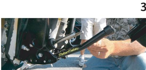
Lower motor very slowly and stop one inch away to make sure the MotorMate End Caps are aligned with the contact points on the motor.
