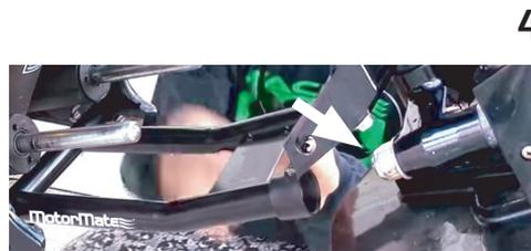
Example of the recessed areas containing the contact points where the MotorMate End Caps secure the motor and where the outboard motor center to center measurements are made.
