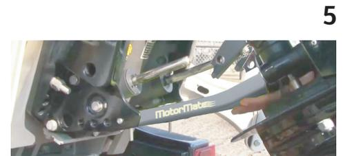
Continue lowering the motor while aligning the MotorMate End Caps with the contact points until the motor is securely held in place.
