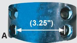
Measure between center to center distance between the contact points.
