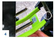
Example of the recessed areas containing the contact points where the MotorMate End Caps secure the motor and where the outboard motor center-tocenter measurements are made.
