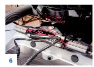
Secure Motor Clips onto hydraulic steering rams on both sides of the motor.
