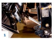
Raise motor and straighten before engaging the MotorMate.
