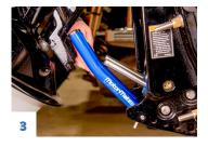
Lower motor very slowly and stop approximately one inch away to make sure MotorMate End Caps are aligned with the contact points on the stern bracket.
